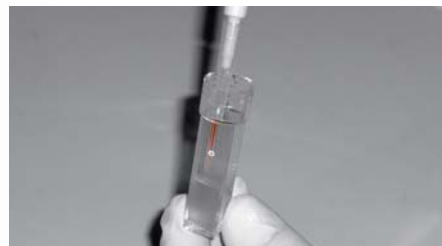
2 Addition of the sample into the cuvette and mixing with capillary or pipette
